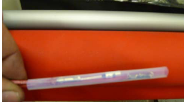
2c: Slide the insulating tubing over the fuse assembly.
