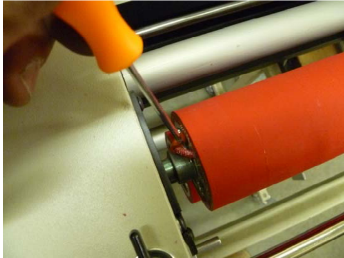
1c: Use the hook to pull the wire out from the left side.
