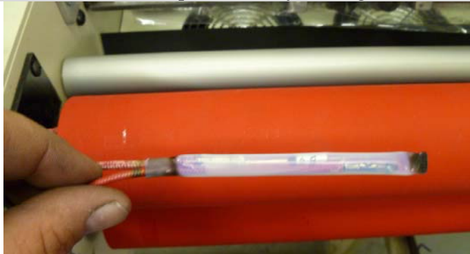
2e: Use the torch to CAREFULLY heat the tube on the opposite end only at the last ¼" until it closes around the wires.
